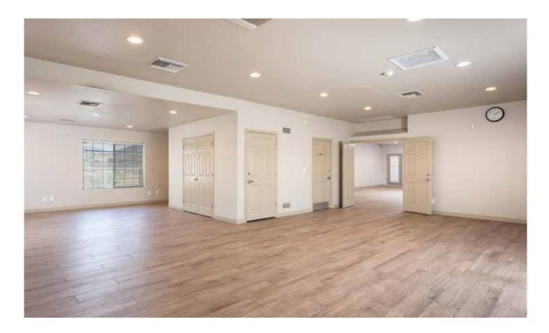
The interior updates were during spring and included a number of items. One update was the flooring, which had previously been a bland generic vinyl floor covering that showed numerous imperfections in the underlying concrete slab joints. The renovation project installed new simulated wood plank ceramic tile, which made the biggest impact on the overall look of the facility.
